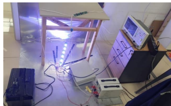
Figure 5: Conducted emission test setup
