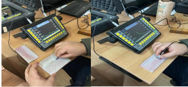
Figure 7. Ultrasonically inspected specimens
