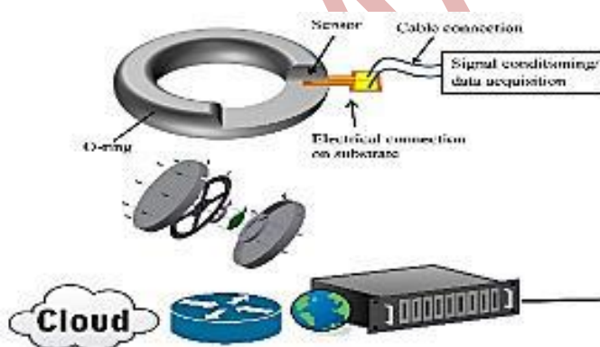
Figure 1. Sensor system based on electrospinning and 3D printing
