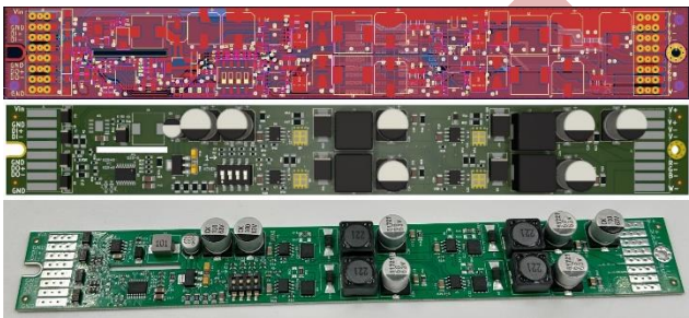
Figure 3. DMX512 Constant current driver
