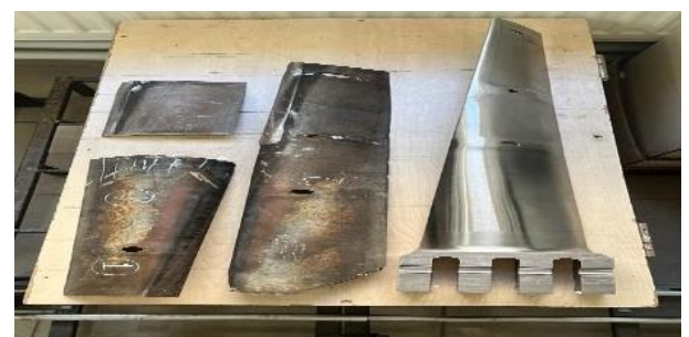
Figure 2. Used and unused steam turbine blades
