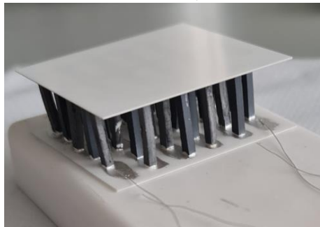
Figure 6. Thermoelectric module where the thermoelectric compounds, silver electric circuit, and output wires can be observed
