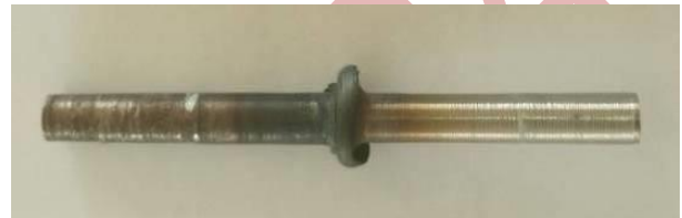
Figure 2. Macrographic view of the welded joint with a rotation speed of 2000 rpm.
