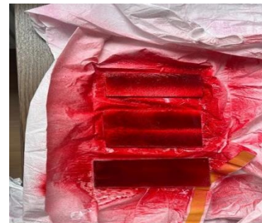
Figure 5. Samples treated with red penetrant
