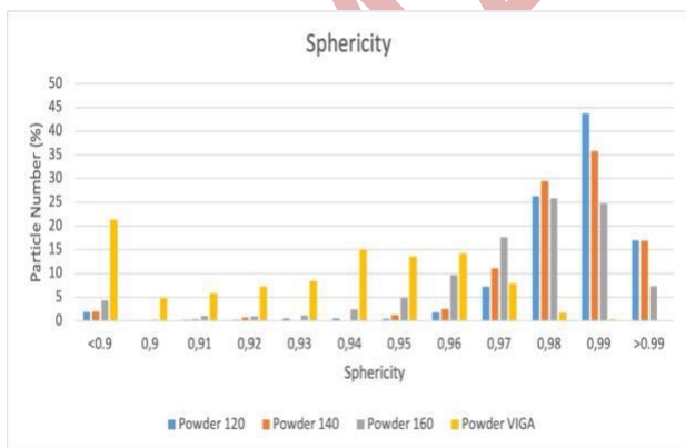
Figure 3. Sphericity of The Powders
